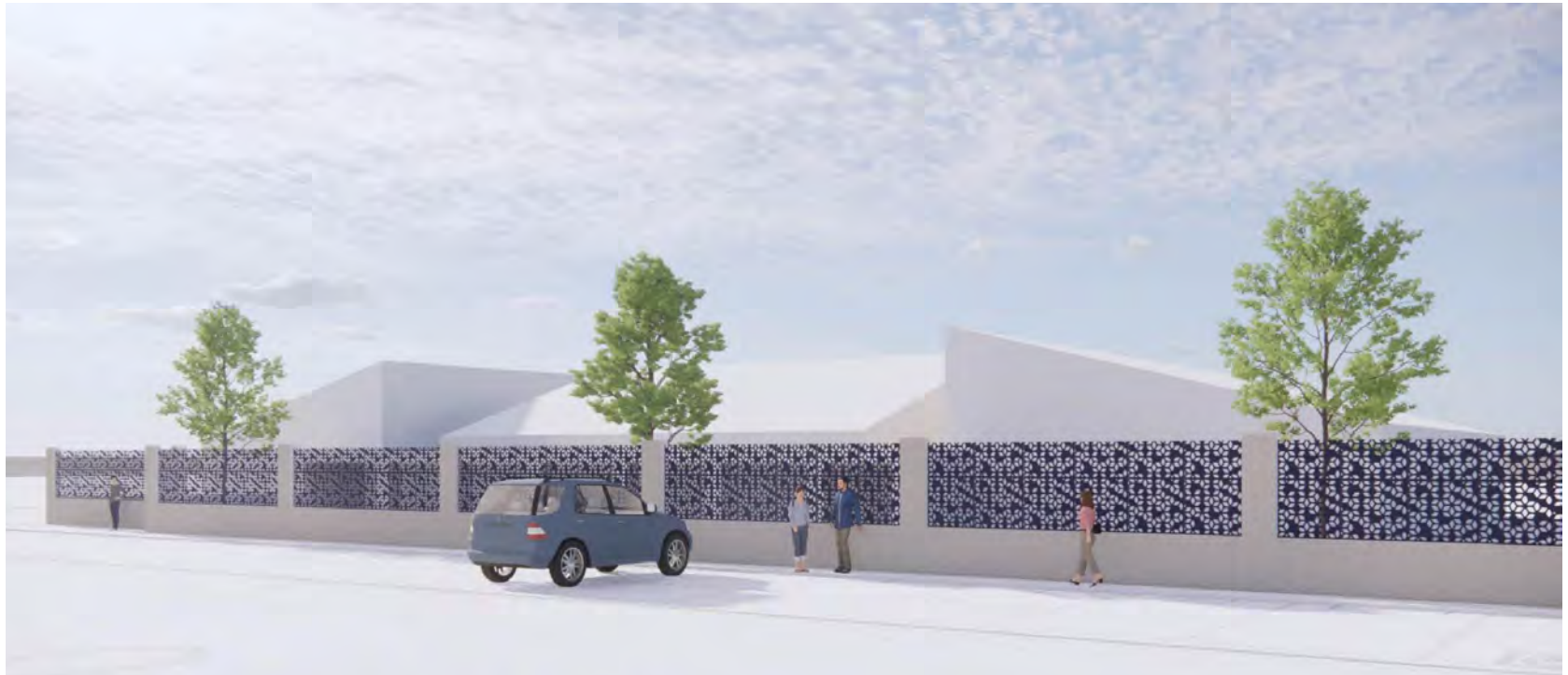
OPTIONS FOR 5'-0" HIGH PERFORATED METAL PANELS ON TOP OF 3'-0" HIGH CMU
